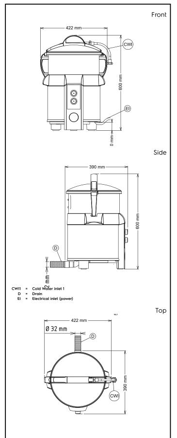
**Electric** Supply voltage: 220-240 V/1N ph/50/60 Hz Capacity: Performance (up to): 80 kg/hour
